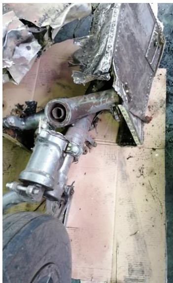
Fig. 15 – Damage to the front landing gear leg.
