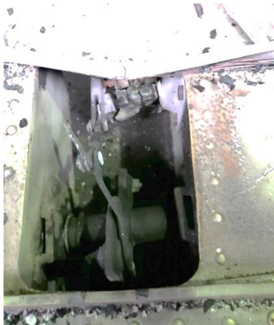
Fig. 17 – Right landing gear leg lock hook
