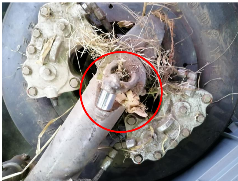
Fig. 19 – Wooden splinters wedged in the left landing gear leg lock eye
