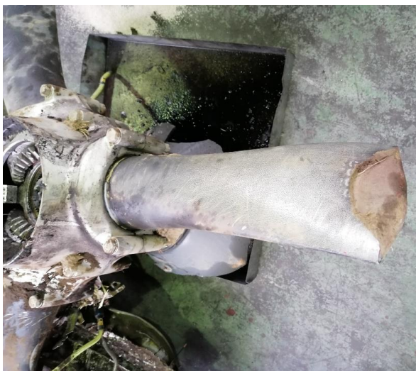
Fig. 11 – Broken propeller blade
