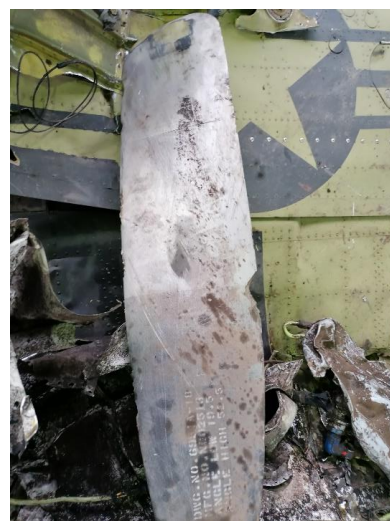
Fig. 12 – Blade with damaged edges
