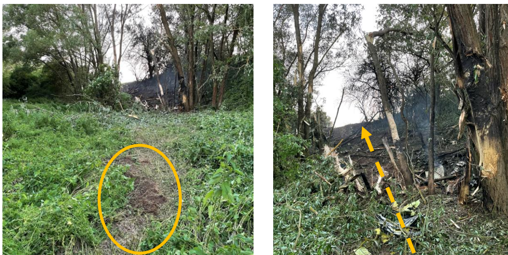
Fig. 10 – Contact of the nose gear wheel tyre with the ground (left) and the point of impact of the aircraft into trees in rising terrain relief (right) with an arrow showing the direction of wreckage movement after impact
