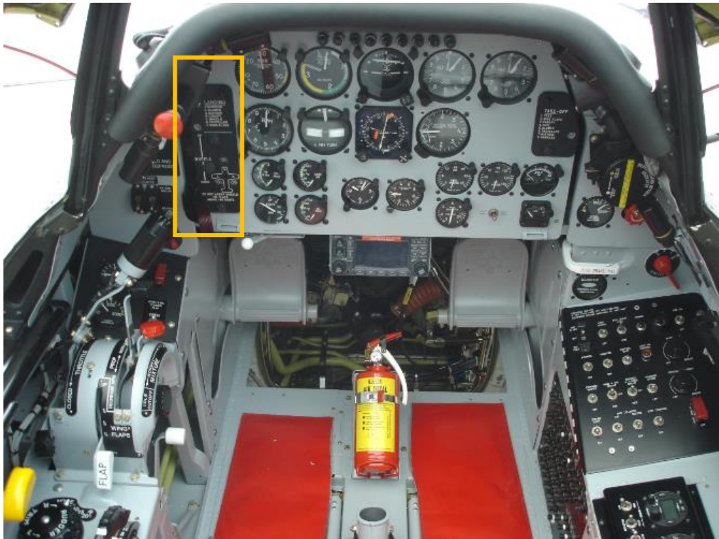
Fig. 7 – Landing gear control in a yellow frame
