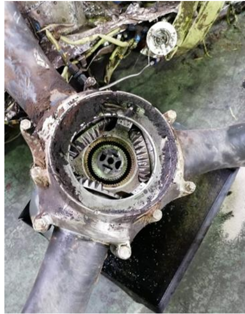
Fig. 14 – Blade setting mechanism in the propeller head
